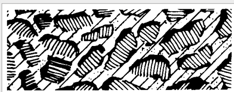
OPEN COAT (1/3 LESS GRAIN THAN CLOSED)
