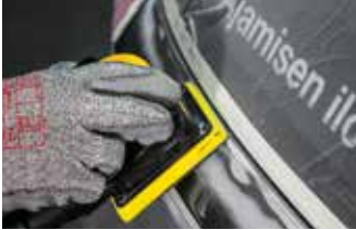
Paint removal and Feather edge sanding
